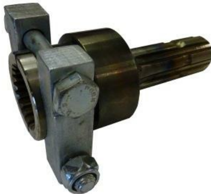
AL00300 - 13/8Z6 male - 25mm plain bore female with 8mm keyway.
