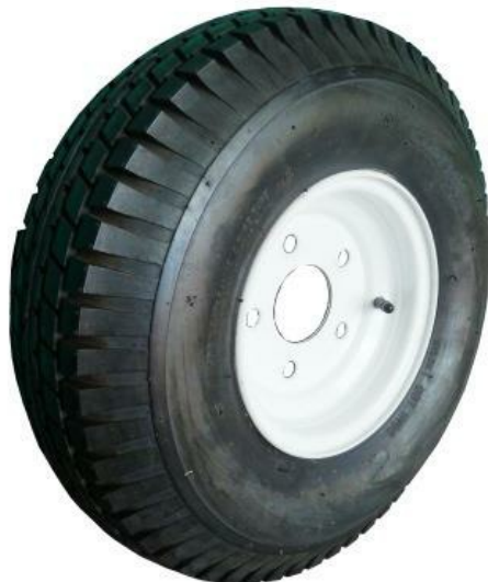
5.00 x 8 - 8 ply highway tyre fitted to a 3.75 x 8 five hole wheel. P.C.D. = 114.3mm (Ford)
