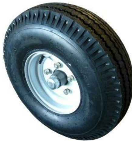
5.00 x 8 - 8 ply highway tyre fitted to a 3.75 x 8 five hole wheel. P.C.D. = 114.3mm (Ford)
